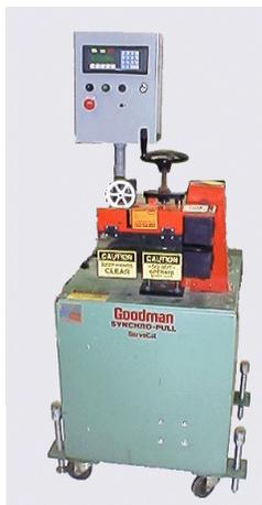
This puller is driven by a Pacific Scientific servo motor and 930 drive.
