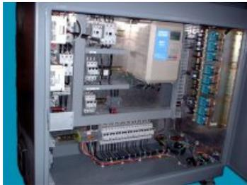
Here you see the nine Solid State Relays mounted on 3 large Heatsinks.
